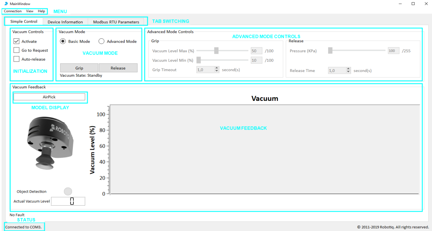
Figure 5.3.1 : The Simple Control tab for the Robotiq User Interface for AirPick Gripper and EPick Gripper.
